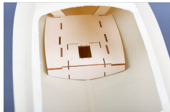
Fig. RC board positioned in hull
