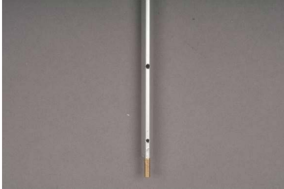
Fig. drill holes for downhaul and boom fitting
