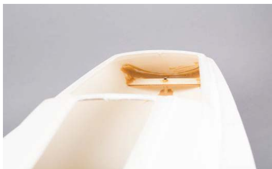
Fig. glued rudder bearing
