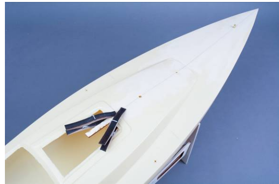
Fig. reinforcing board in position
