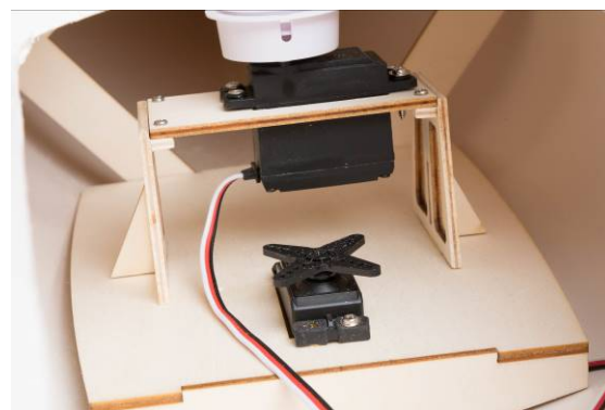
Fig. Sail winch frame on RC board
