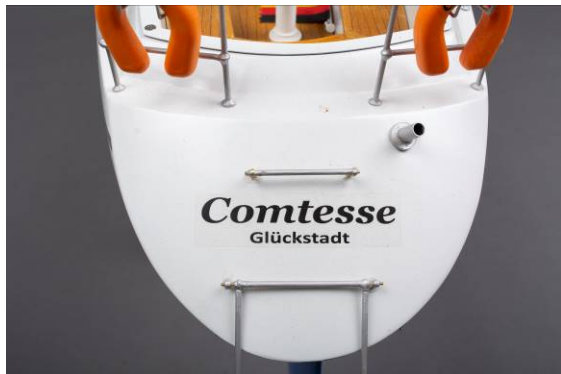
Fig. bathing ladder folded down, additional rung
