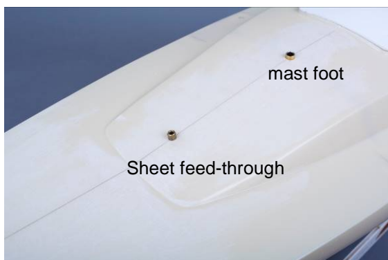
Fig. sheet feed-through jib sheet and mast foot
